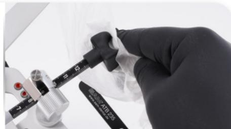
*For the screw thread of the cap nut you can use any kind of lubricant, e.g. silicone spray for straight/contra-angle hand pieces.*
