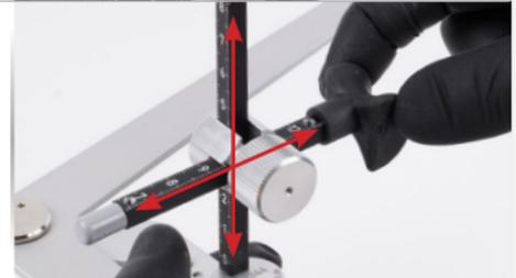
*Finely adjust the resistance by loosening / tightening the polyamid screws.*
