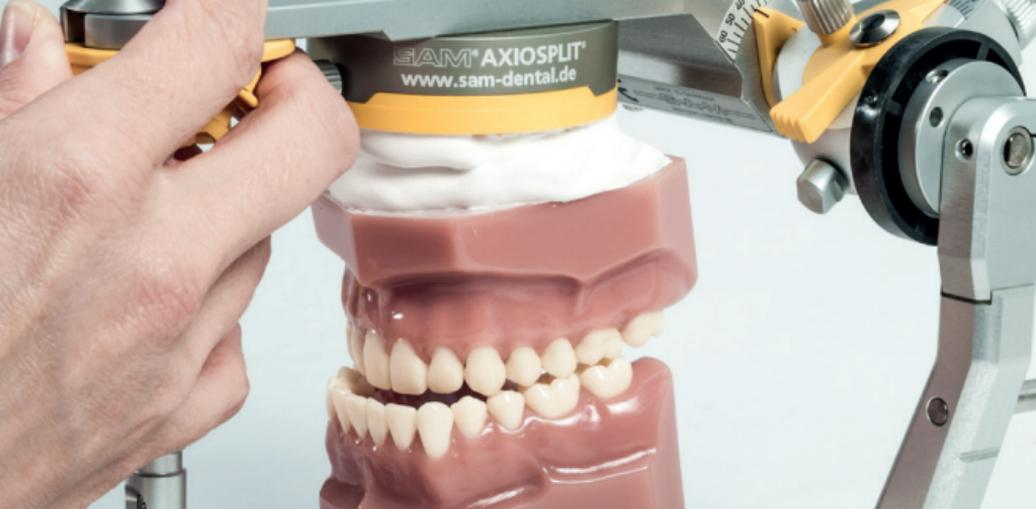
*If colored Bennett guides are used (here the green one), the guide rings enable a fast protrusion movement without changing the inserts with sideshift.*
